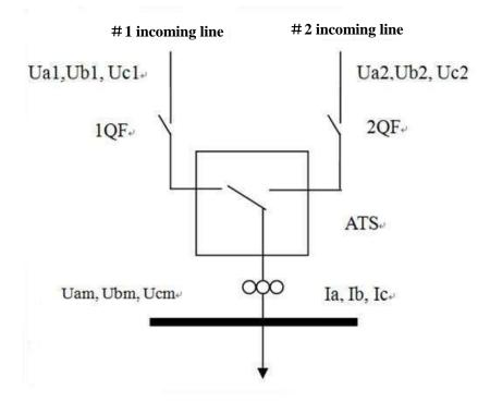
1Ua1, Ub1, Uc1: three-phase voltage of incoming line 1; Ua2,Ub2,Uc2: three-phase voltage of incoming line 2; Uam, Ubm, Ucm: three-phase voltage of bus; Ia, Ib, Ic: three-phase current of bus;1QF, 2QF: switch of incoming line 1 and 2 ,respectively. Principle of operation: For dual- circuit substation transformer outputs, one of them is connected to low-voltage AC power supply bus through dual power automatic
