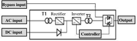
Principle Block Diagram of UPS Special for Electric Power
