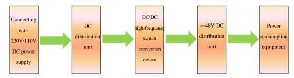
Principle of operation: Through high-frequency switch DC conversion technology, convert  $220V \setminus 10V$  DC voltage input from the DC power supply to 48V DC voltage output.
